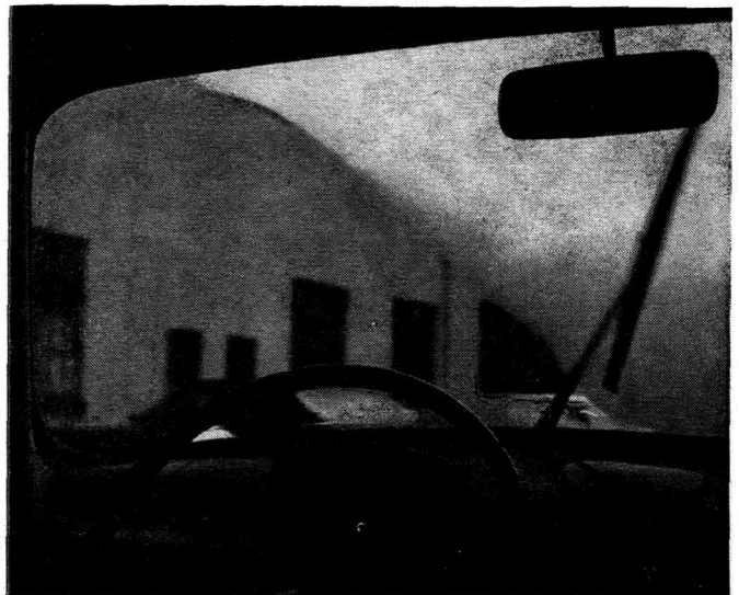
Even at maximum performance, the defroster/defogger on the Subaru cleared no more than this wedge-shaped piece of the windshield, leaving the rest of the car entirely fogged in
