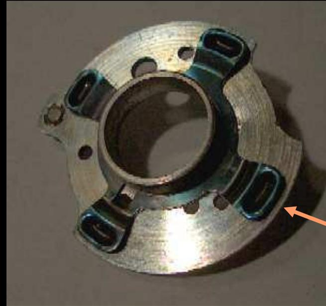
6. Start with the flat 4 sided part of the bearing race, then place the cupped 4 sided part of the race making sure the tang rests in the smaller of the two larger holes in the bright colored plate. See picture above.
