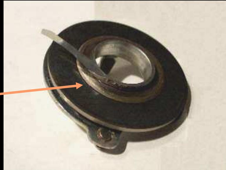
**11. Once you have all the shim in place, use a razor blade to trim the excess and fold the shim stock above the dark plate over onto the plate (do not cut it off).**
